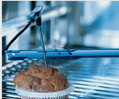
5. When loading the SelfCookingCenter® with **products of different sizes**, e.g., different pieces of meat, it is generally best to insert the probe into the smallest product. When using cooking processes followed by holding stage (Overnight Roasting, Braising, or Overnight Boiling), make sure that the holding stage is long enough that the larger products will reach the desired core temperature as well.
