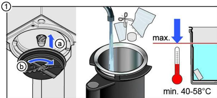
Attach the Pacotizing® blade and spray guard, fill the Pacotizing® beaker to the maximum fill line with 105 - 135°F warm water, add a Pacojet Cleaning Tab, attach the Pacotizing® beaker and protective beaker, start cleaning process.
