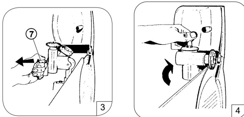
To sharpen, first turning the switch in on position, so that the knife turns, the slowly rotate the lever which lets both stones go in contact with the knife; sharpening and trimming are made in same time fig. 5
