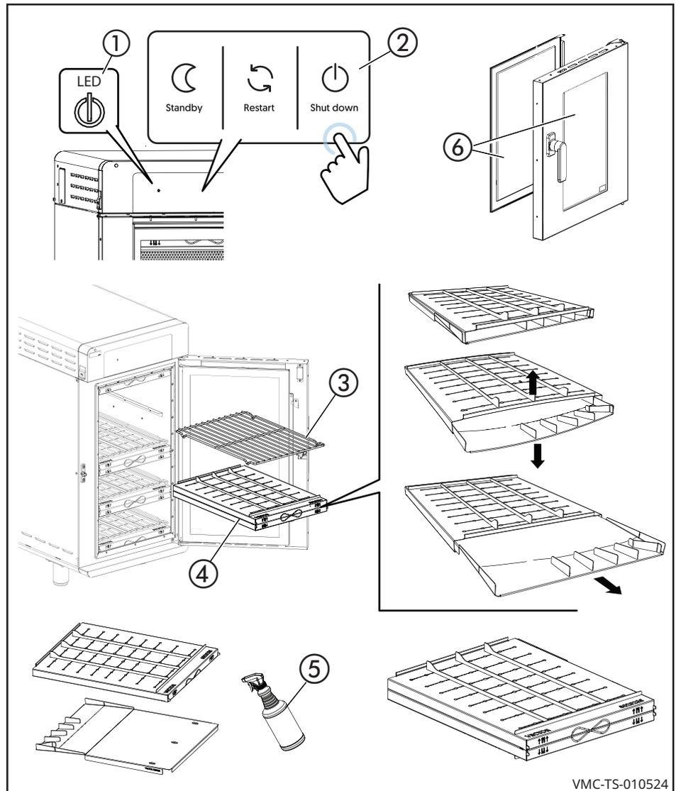
**NOTE:** Make sure the jet plates are installed correctly. The nozzles on the jet plates should be pointing towards the food.
