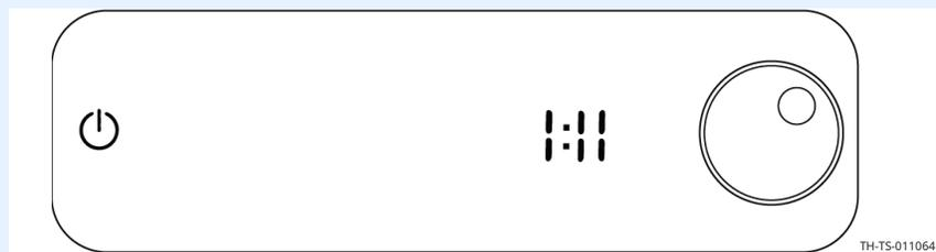
7. Power failure (PF) displays.
