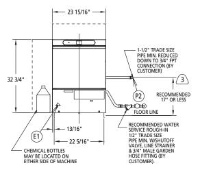
**NOTE:** Certain materials, including silver, aluminum and pewter are attacked by sodium hypochlorite (liquid bleach) in the chemical sanitizing dishwasher mode of operation. Water hardness must be controlled to 3 grains OR LESS for best results.
