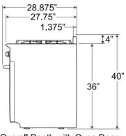
Overall Depth with Oven Door in fully open position - 44.5"
