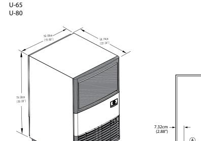
**Installation Note** - There is no minimum clearance required, however recommended clearance for top, sides, and back is 5" (12.7 cm).
