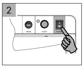
Flip "ON/OFF" switch to "ON" position
