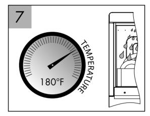
Final rinse temperature should be a minimum of 180°F/82°C during the final rinse. (140°F/60°C for low temp. model)
