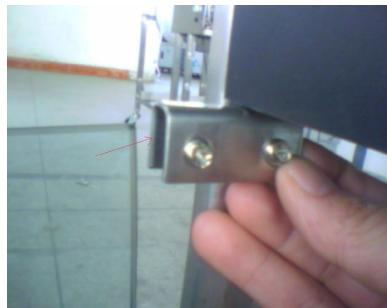
3. Place the left side top door hinge assembly into the upper frame left hole slot and proceed to slide and insert the complete glass door into the top door hinge. Please note the arrow direction in the figure above. Once in place slide supplied gaskets in between door hinge assembly and glass door making sure white gasket is in behind door hinge with screws and tighten loosely.
