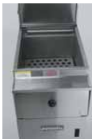
Vessel is 16 gauge 317 alloy stainless steel to withstand stronger concentrations of salt in the water
